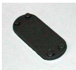
(1) Driver's View Port Bolt Detail
