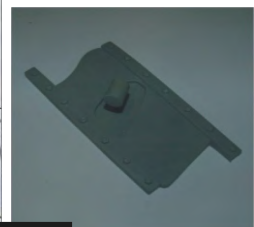
Figure B - Periscope Guide Rail Assembly Drill a 1/4" hole in Periscope Guide Rail and insert the leg of Upper periscope. Secure with Super-glue.
