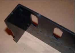
Dry fit the Equipment Shelf into the lower hull. Use one edge of the Equipment Shelf as a brace for the 12volt battery. When satisfied with the location, apply adhesive to mount the unit to the lower tank hull.
