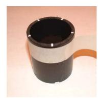
**Step 13:** Gear Spacer Assembly: Center the Gear Spacers onto the Spacer Tubes, opposite the cog grooves. Glue the Spacer to the Gear with ABS adhesive.
