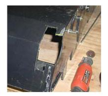
Step 7: Mount Installation: Use ABS adhesive to glue the Outside mount on top of the hull cut, flush with the edge. Glue the Support Mount against the inside of the Outside Mount. Repeat for the other side.
