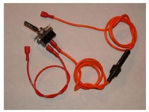
The toggle switch is to be mounted on the Equipment Shelf. Select a position that can be reached from the open engine grille, located on the upper hull. Drill a 3/8" hole through the Equipment Shelf and insert the toggle switch from the bottom of the shelf. Secure the toggle switch with the mounting nut.
