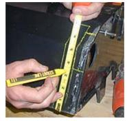
Step 6: <u>Locating Track Motors, Continued:</u> Mark 1-1/4" from the bottom hull angle plate. Draw a line from the 1-1/4" mark. Repeat for the other side.
