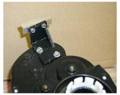
**Step 10:** Track Motor Installation: Push the Track Motor into the cut-out hole in the hull. The mount on the front of the Track motor will click into the Outside Mount hole, which was installed in Step 7.
