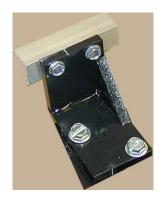
Step 9: <u>Attach Motor Mounts to Motor Housing:</u> Attach the Rectangle Plates to the Track Motor housings, using #11 screws. Use the existing holes in the track motor housings.
