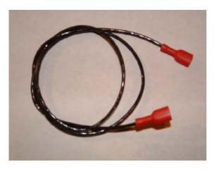
Step 4: Wiring for Motor Harness: Cut two pieces of the black and red wires, each 24" long. Attach a female connector to each end of the four wires. Use electrical tape to connect the wires into two pairs, each with one black and one red wire. Each pair of wires is to be connected to a motor, with the other ends connected to the speed controller(s).
