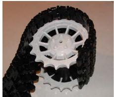
Step 17: <u>Drive Sprocket Installation:</u> Slide the Drive Gear Assembly onto the drive gear axle. Slide the drive gear axle through both Track Motors. Press the backside of the Drive Gear Assembly onto the Track Motor teeth. Attach a push nut to each side of the drive gears and secure the axle in place.
